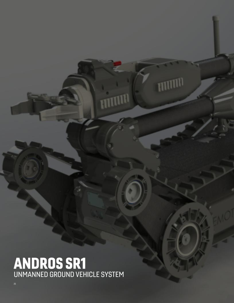
The Andros™ SR1 is a lightweight, one-man portable, unmanned ground vehicle system developed for missions requiring first look, fast reconnaissance, tactical response, and render safe for EOD operations.
